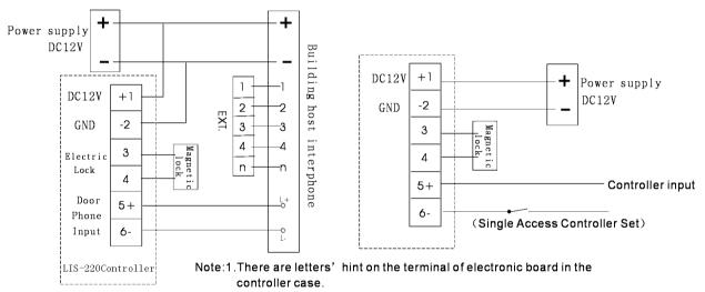
2.If the voltage is lower than 6V, it can't tough off the opening signal the door will be in the locking state.
