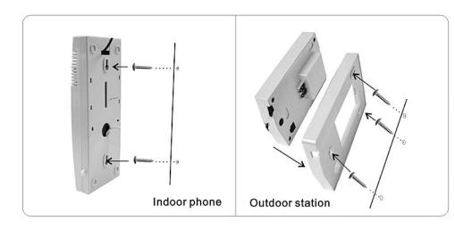
The optimum height of the indoor phone and outdoor station for installation is  $145\sim160$  cm from the ground(This data provides to consult only).
